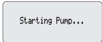
The pump will review the program, lock level, AutoLock setting, air detector status, time, and date.
